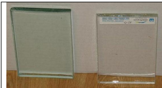
Picture 1 Above (Left) Standard Glass, (Right) Low Iron Glass
